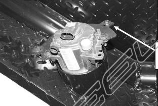
(Fig 19) Fog light with Bracket installed
