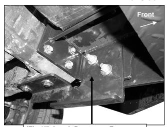
(Fig 17) Attach Bumper to Frame Bracket and Support Bracket, (driver/left side pictured from below)
