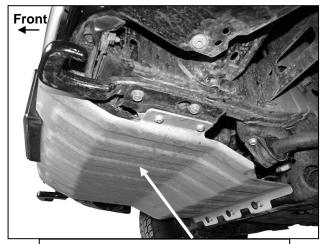
(Fig 4) Remove skid plate if equipped
